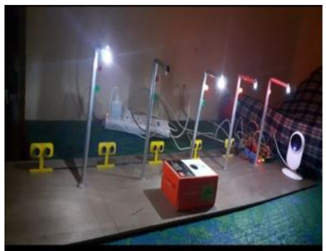
Figure 5: Red LEDs are glowing as alert system for upcoming vehicles.
